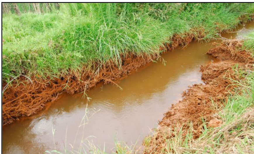
Plate 6 Examples of Fe-(orange) and Mn-oxide (black) precipitation as concentric scaling in pipe (left) and as 'Yellow boy' in ditch (right) (photo at left J Davies; photo at right W Basson).
