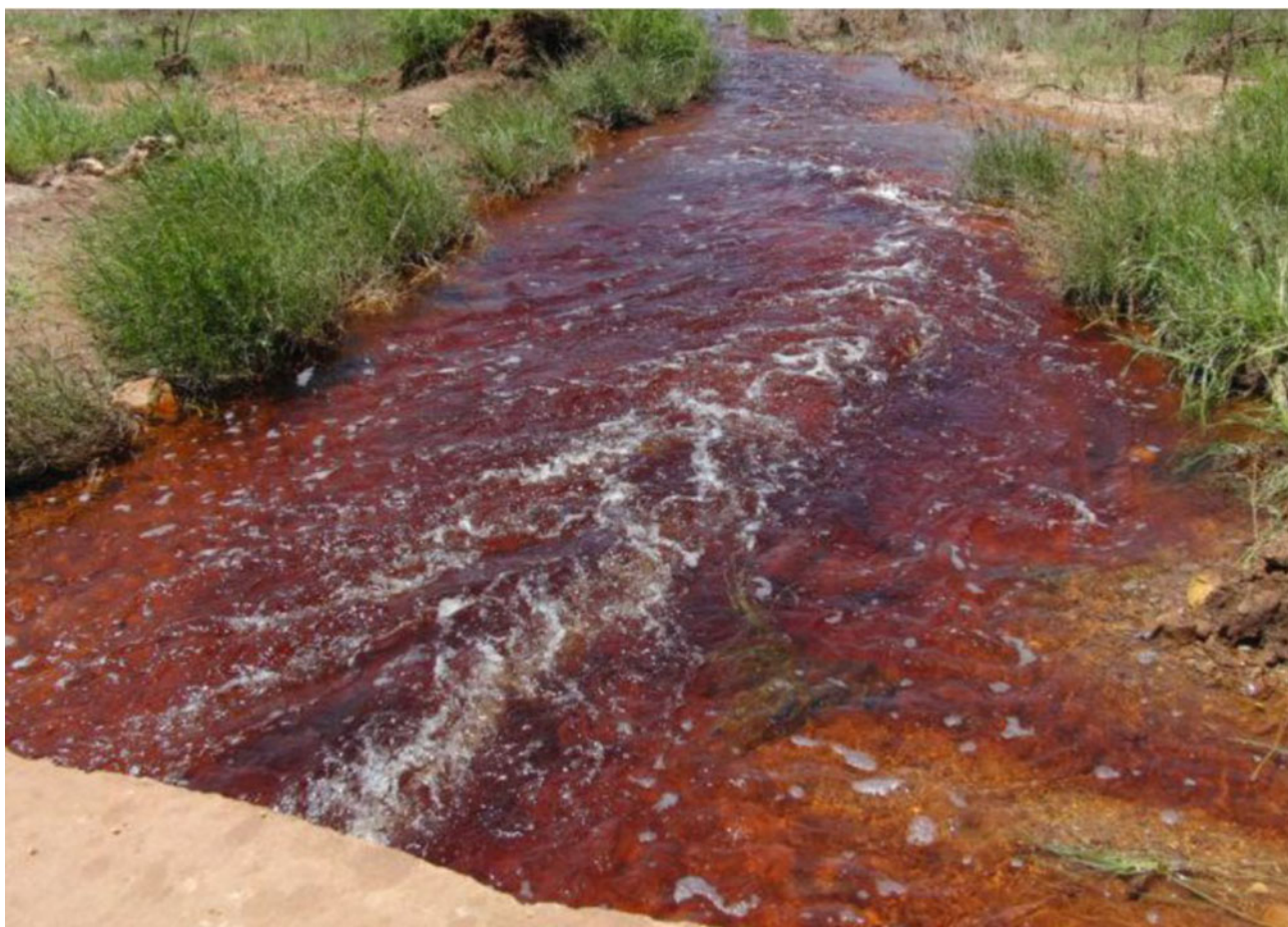
Discharge in the Riet Spruit at its intersection with the Malmani Road; note the red colouration of the water due to dissolved ferrous iron ( \text{Fe}^{2+} ) indicative of a strong acid mine water presence as revealed by the following field values: pH = 2.3, SEC = 410 mS/m, ORP = 254 mV (photo P Hobbs, date 12/01/2011)
