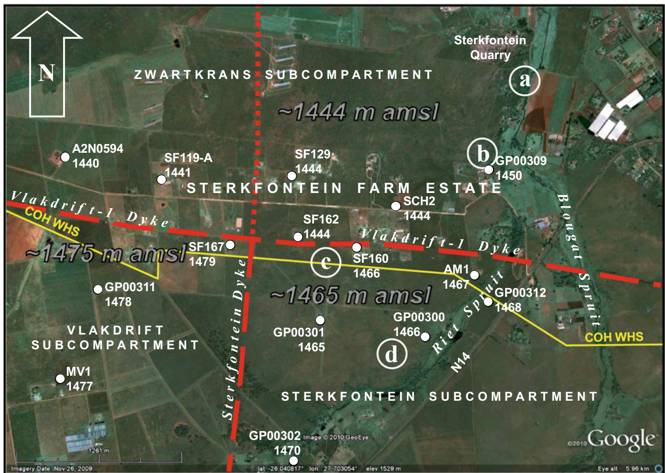
Fig. 18 Elucidation of hydrological, geological and hydrogeological aspects along the southern boundary of the COH south-west of Sterkfontein Quarry; circled localities labelled 'a' to 'd' mark the position of significant grike features, and italicised values indicate the
