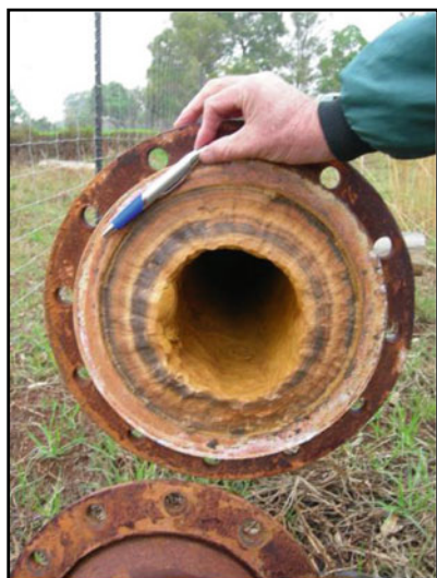
Plate 6 Examples of Fe-(orange) and Mn-oxide (black) precipitation as concentric scaling in pipe (left) and as 'Yellow boy' in ditch (right) (photo at left J Davies; photo at right W Basson).
