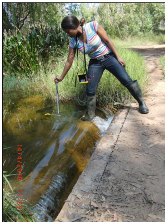
Plate 8 View of synoptic discharge measurement with current meter in progress at site F11S12, showing both the relatively ‘clean’ cross-sectional area of flow (from bottom left to right foot of observer) and the laminar nature of flow over the crest of the weir
