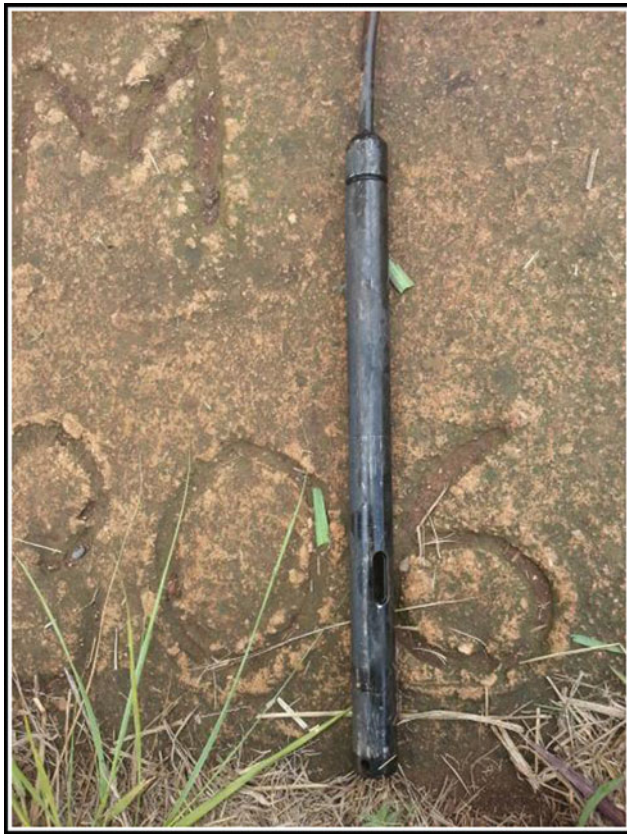
Plate 8 Data logger (length ~20 cm) from monitoring borehole GP00305 completely coated with black iron sulfide (FeS) precipitate on stainless steel instrument (photo N. de Meillon)
